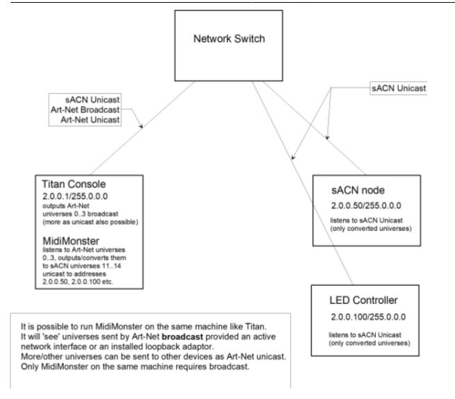
The question arose if the additional computer could be spared and if MIDIMonster could be run on the same machine Titan runs on. As explained in the section above this does **not** work with sACN - the external nodes see that MIDIMonster sends something but the values are always 0. I suspect this is due to some fancy network routing problem: two programs attempting to send on the same port and on the same machine, AND one program trying to listen to the other.
