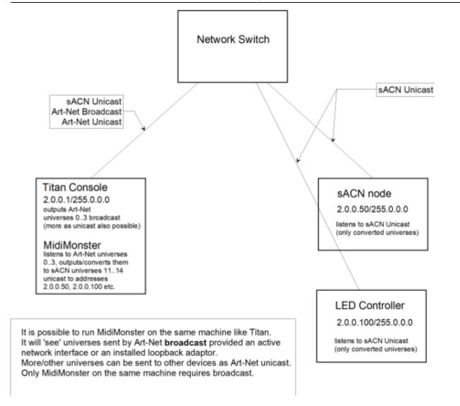
The question arose if the additional computer could be spared and if MIDIMonster could be run on the same machine Titan runs on. As explained in the section above this does **not** work with sACN - the external nodes see that MIDIMonster sends something but the values are always 0. I suspect this is due to some fancy network routing problem: two programs attempting to send on the same port and on the same machine, AND one program trying to listen to the other.
