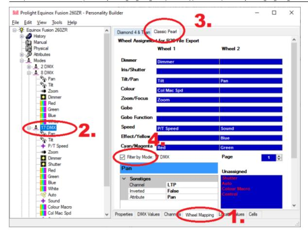
In the righthand area you can now drag and drop each attribute, in order to move it to another bank and wheel. Usually the suggested mapping is a good starting point. The most important thing is to move attributes from the 'Unassigned' area (bottom right) onto a valid blue rectangle (defined by Wheels and attribute group). Also using the Page select box with arrow buttons you can toggle to more pages. My result looks this:
