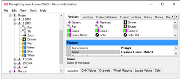
• the **25 DMX** mode contains the sections Cell Master, Cells, and Compatibility Attributes (here empty) - this is a mode which uses cells, and thus cannot be exported as R20.
