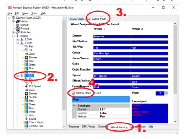
In the righthand area you can now drag and drop each attribute, in order to move it to another bank and wheel. Usually the suggested mapping is a good starting point. The most important thing is to move attributes from the 'Unassigned' area (bottom right) onto a valid blue rectangle (defined by Wheels and attribute group). Also using the Page select box with arrow buttons you can toggle to more pages. My result looks this:
