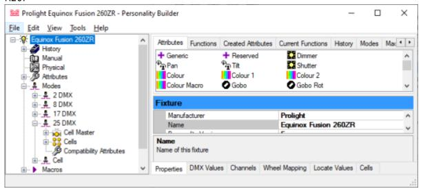
• finally the **Cell** mode is the one which is only referenced in the 25 DMX mode. proof for this is the **Hidden** attributes set to true: left, click on the mode **Cell** itself, and in the properties section (bottom right) you'll find Hidden set to True:
