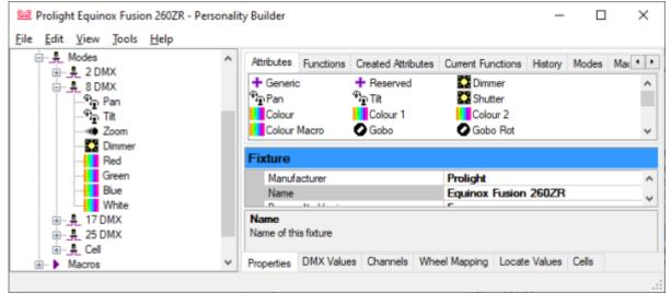
• the **25 DMX** mode contains the sections Cell Master, Cells, and Compatibility Attributes (here empty) - this is a mode which uses cells, and thus cannot be exported as R20.
