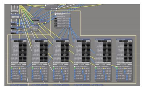
This part is pretty much straight-forward: each one of the six screens which are standing in mediaspinners on the ground is represented by its own screen fixtures so that each one can be loaded its own model (again, distinct by the UV mapping), and can be controlled, as per the y roation, via Artnet from the Mediaspinner controller.
